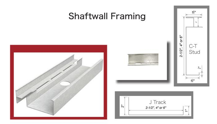
The two primary framing components in Shaftwall framing is the liner board and C-T Studs and J Tracks, manufactured from galvanized steel that meets the requirements of ASTM A 653 and A 924.
