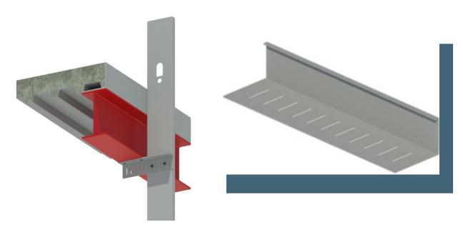
Outrigger Slide Clips are used for horizontal surface applications and offers the highest capacity of any surface connection clip. The Outrigger comes in 18" and 12" lengths and can be field cut to shorter lengths if needed. Simple and fast to install which saves time and money. One clip fits all stud sizes and there is no right or left hand clips.
