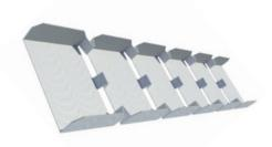
Flex Track is the easiest and most cost efficient method to build curved walls, ceilings or bulkheads. Flex Track bends both ways to create non load-bearing curves and openings, including wavy ceilings, barrel vaults, arches and columns. Flex Track can be used with wood or steel studs.
