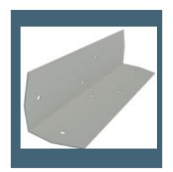
Bridging Clips are used for the installation of bridging channel for both wind load and combined wind and axial load bearing applications at every location where a carrying channel meets a steel stud. Four fasteners (#8 or #10) per clip are used in pre-punched (0.160") holes. The clips can be used on the inside or outside of stud.
