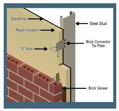
The unique design allows for use with all steel stud systems from 3-5/8" to 8", with all exterior sheathing and insulation products.
