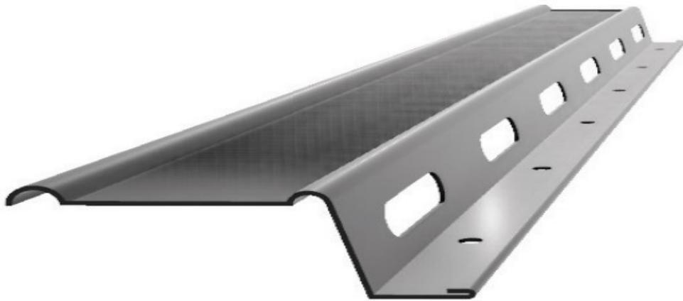
Resilient Channel is a cost effective product used on steel and wood studs, and LSF and wood joists as an assembly for achieving specified STC (sound transmission classification) ratings. The pre-punched slots or holes in the metal web provide resiliency to reduce sound transmission through the steel. Resilient Channel is also an economical framing member used for leveling the underside of wood joists in basements and used for drywall attachment.
