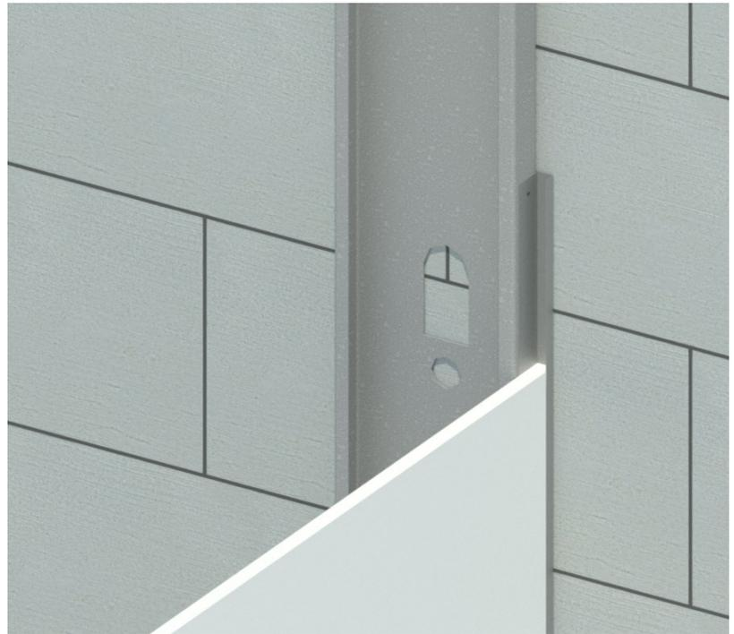
Metal J Trim provides edge protection at window and door openings and where wallboard butts against concrete or other materials. J Trim is installed prior to wallboard installation and finishing compound is optional. J Trims are used with 1/2" or 5/8" wallboard and are available in 8' and 10' lengths and are packaged in 20pcs/ctn.
